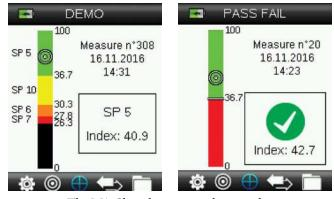
The WA Clean has two working modes: Cleanliness measurement (left) or PASS/FAIL (right).
